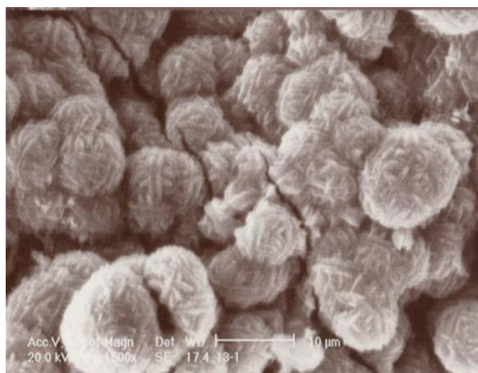
Figure 9: SEM micrograph of zeolite HS membrane preparation of kaolin source
